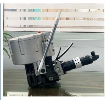
Specially optimized for 19mm wide steel straps, it ensures a perfect match between the packing straps and the equipment, avoiding problems such as loose locking or insufficient tension caused by size mismatch.
