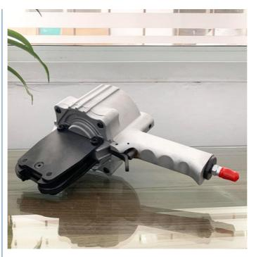
1, excellent performancePatented locking technology, clamping force up to 15000N, 1.5 times that Optimized gas path design to maintain stable output at 0.49-0.63Mpa working pressure
