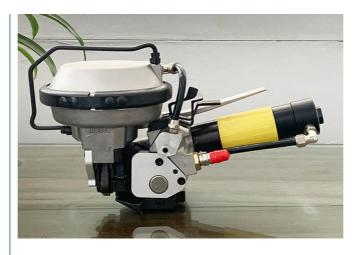
Its maximum pulling force can reach 3000N, ensuring that the strapping is firm and reliable, especially suitable for the fixation and transportation of heavy goods. The equipment adopts pneumatic drive mode, operating pressure range of 0.4-0.6Mpa, strong power and stable operation, can efficiently complete the bundling task, while reducing the labor intensity of the operator.
