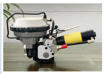
First of all, L-KZ16 pneumatic integrated strapping machine has a strong strapping capacity, the maximum tension of up to 3000N, can firmly tie a variety of heavy goods, to ensure the safety and stability during transportation and storage. Its applicable air pressure range is 0.4-0.6Mpa, simple and efficient operation, can quickly complete the bundling task, significantly improve work efficiency.
