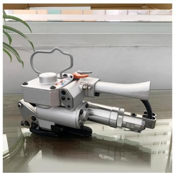
The pneumatic baler is widely used in PET and PP two kinds of material packaging belt, the width of the packaging belt range between 13-19mm, the thickness is between 0.4-1.2mm, this wide applicability makes it able to cope with a variety of different packaging scenarios and needs.
